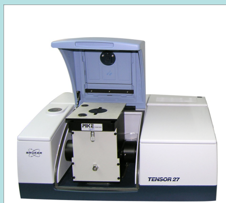
圖2: 德國紅外線光譜儀 Bruker Tensor 27 FTIR Spectrometer, Germany
